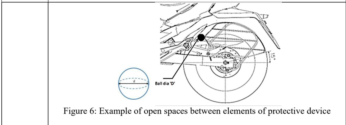
Figure 6: Example of open spaces between elements of protective device
