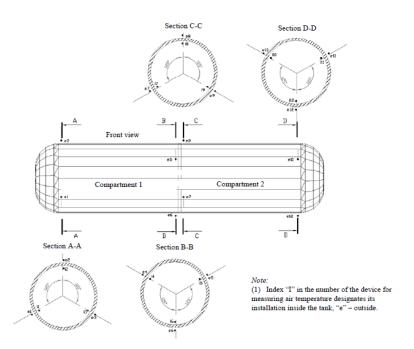
(c) If the tank has several compartments, the points of measurement shall be as follows for each of the two end compartments, at least the following:
