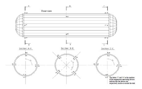
(b) If the tank has two compartments, the measurements shall be made at least at the following points:
