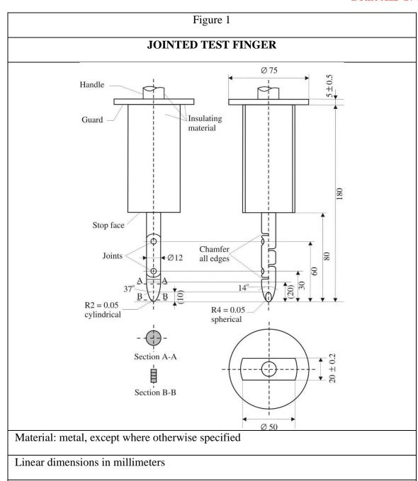
Tolerances on dimensions without specific tolerance:
